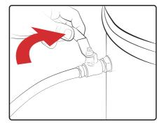
Unless you know that your vacuum pump has a built-in one-way 'check valve', always close the vacuum valve that connects the chamber to the vacuum pump before switching the pump off.
