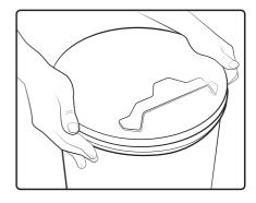
Press down firmly on the lid to make sure it is well seated into the seal.
