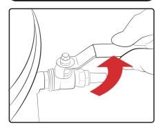
To let air back into the chamber, turn the re-pressuring (inlet) valve on the degassing chamber counter-clockwise into the open (inline) position.
