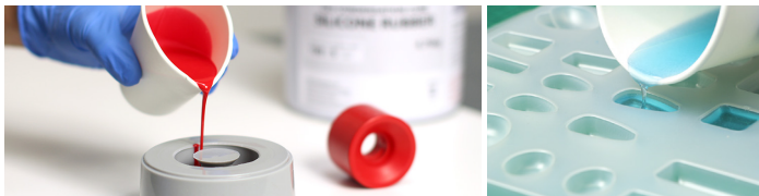
Pigmented PX90 being poured into a CS25 Condensation Cure Silicone mould
